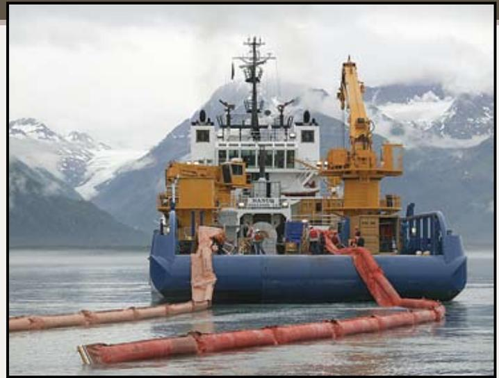
"Nanuq" - an ice class vessel built specifically for spill response in the Arctic.
